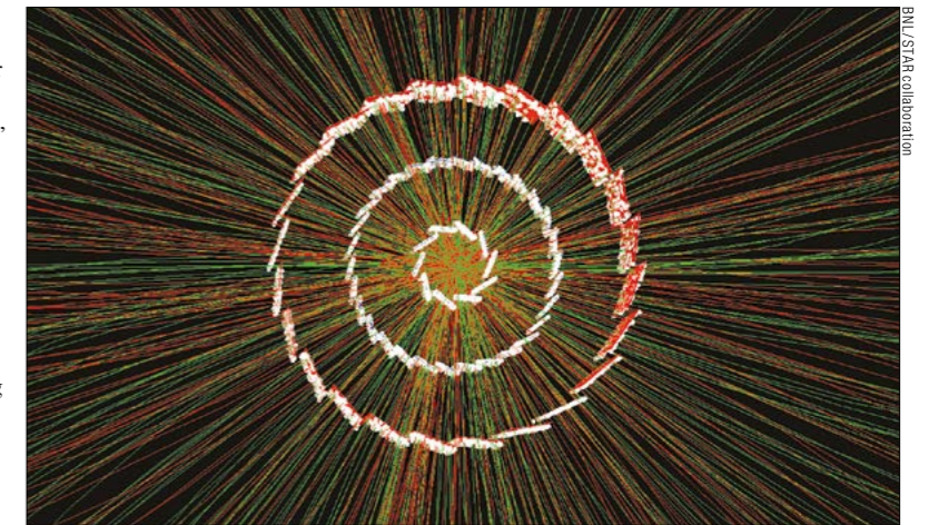
A gold–gold collision recorded by STAR with the MAPS pixel detector (two most inner layers) and one layer of silicon-strip detector (outer layer). The white points show the measured hits that were used to reconstruct charged particle tracks (red and green lines).
