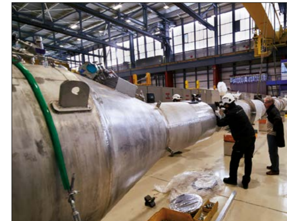
Fig. 4. The ARIA modules for purifying liquid argon being tested at CERN.
